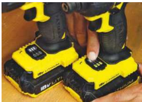
▲ Indicators on both units show the battery power status
